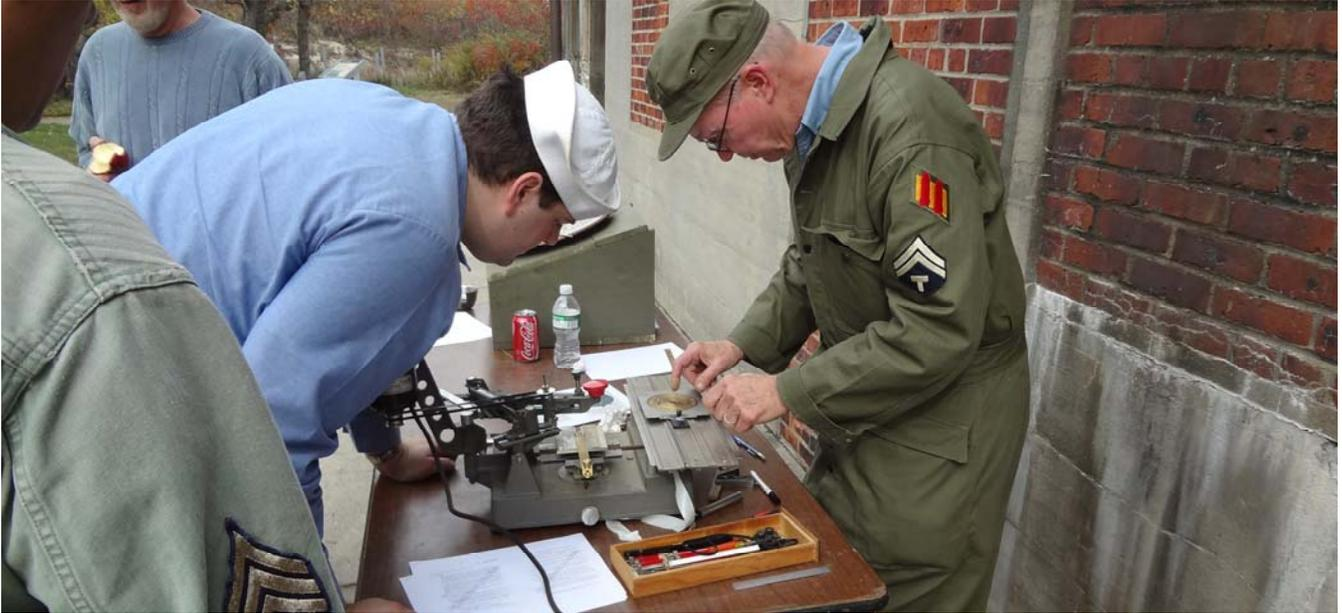
Below, T-5 Komorowski and BM2 Kaiserman use a "lettering machine" from the 1940's to mark the scale with numbers and "Target Arm Scale" as the original Arm would have looked. T-5 Komorowski used new brass bar stock to make the arm, and then the instrument below marked the arm scale proper with its measurements and lettering. The left corner of the photo shows part of the Wind Component Indicator.
