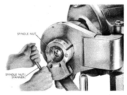
Figure 25 — Removing Obturator Spindle Nut
