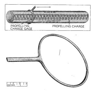
Figure 85 — Propelling Charge Gage (6-inch Gun M1900, 03, 05) (24-4-3249A1)
