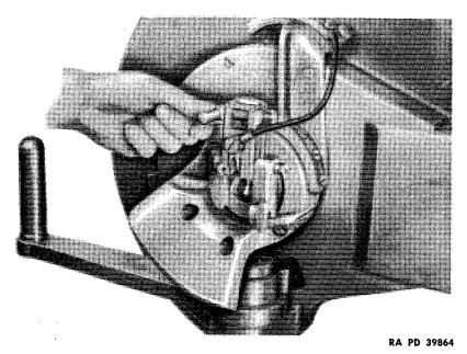
Figure 15 — Opening Firing Mechanism Slide To Remove Primer
