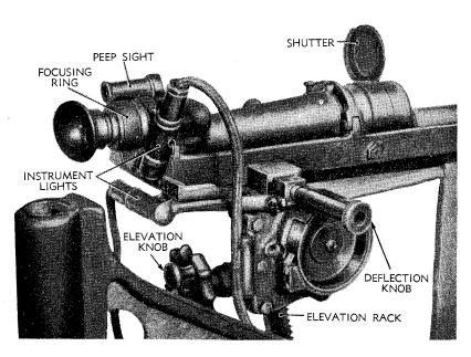
Figure 46 — Telescope Mount M1904MIA1 With 3-inch Telescope M1904MI — Side View
