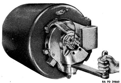
Figure 12 — Operating Lever Pulled To Turn Breechblock
