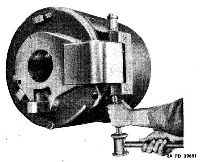
Figure 37— Driving Out Hinge Pin
