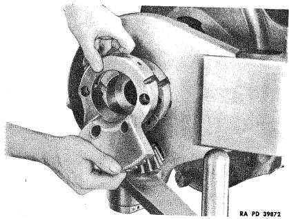
Figure 28 — Disassembling Gear Segment
