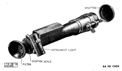
Figure 48 — 3-inch Telescope M1904 — Side View
