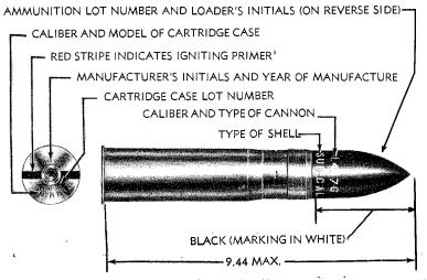
Figure 60 - 1.457-inch Subcaliber Shell RA PD 5290A
