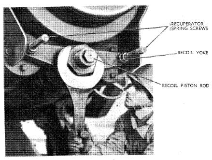
Figure 42 - Adjusting Recoil Piston Rod M1900
