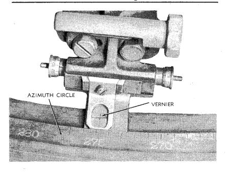
Figure 11 — Traversing Vernier M1900
