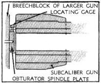
4. SUBCALIBER GUN IS IN CORRECT ADJUSTMENT IF LOCATING GAGE IS PUSHED UP SNUCLY AGAINST OBTURATOR SPINDLE PLATE WHEN BREECHBLOCK IS CLOSED
