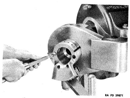
Figure 27 —Removing Segment Gear Screws
