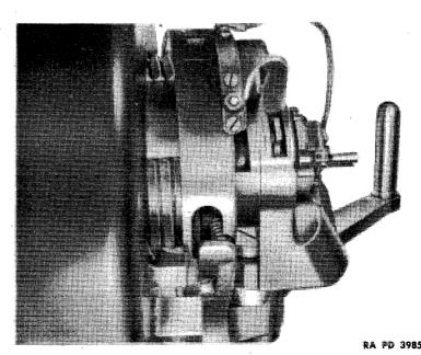
Figure 5 — Tooth on Operating Lever Gear Pushing Breechblock
