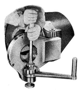
Figure 36 - Removing Operating Lever Pinion - Nut Removed
