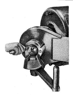
Figure 24 —Removing Spindle Nut Screw
