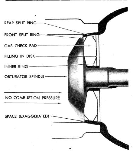
Figure 6 — Obturator in Normal Position
