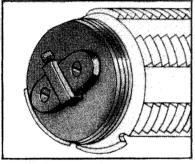
3. PLACE LOCATING GAGE ON OBTURATOR SPINDLE PLATE (LEAVING SPACE BETWEEN GAGE AND PLATE)
