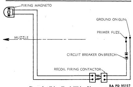
Figure 8 — Firing Circuit Wiring Diagram
