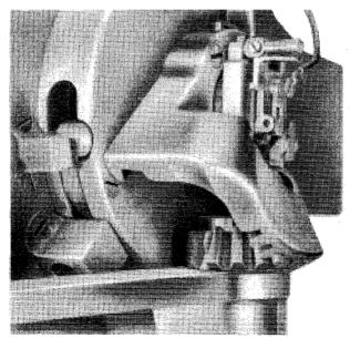
Figure 3 - Closed Position - Close-up of Segment Gear
