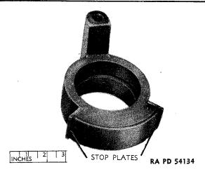
Figure 102 - Rear Adapter (63-7-21B) W/Stop Plates (63-7-21A)
