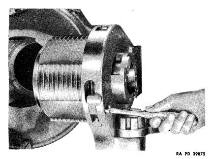
Figure 31 — Removing Breechblock Lock Screw
