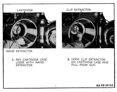
Figure 100 — Cartridge Case Removal (6-in. Gun M1903A2 Shown)
