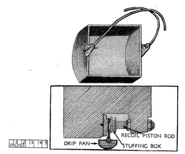
Figure 96 — Stuffing Box Drip Pan (Model A) (15-3-2)
