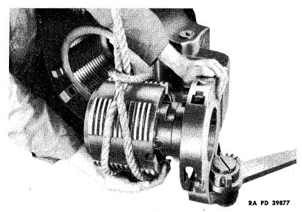
Figure 34 - Removing Breech
