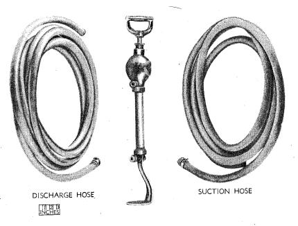
Figure 76 - Force Pump (Plumber's (11-P-430)
