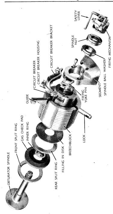
Figure 20 — Breechblock Mechanism — Exploded View
