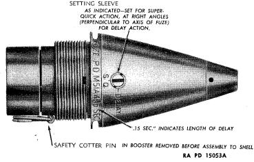
Figure 59 — Point-detonating Fuze M51A4, w/Booster M21A4
