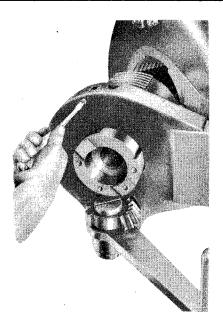
Figure 29 - Removing Breechblock Guide Screw
