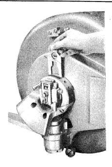
Figure 22 - Removing Firing Mechanism Yoke
