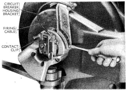
Figure 21 — Firing Contact Removal
