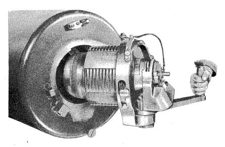
Figure 14 — Breechblock Starting To Swing on Carrier
