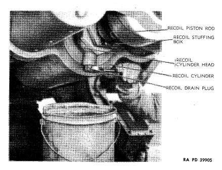
Figure 41 — Emptying Recoil Cylinder M1900
