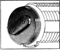
ASSEMBLE OBTURATOR SPINDLE PLATE ON OBTURATOR WITH SECURING SCREWS
