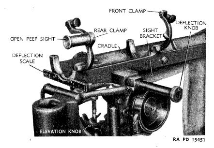
Figure 45 — Telescope Mount M1904MIA1 — Rear View
