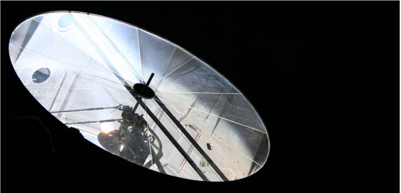
The searchlight is shown below with its light extinguished. The mirror is much more evident in this shot. These lights burn with such intensity that the parts begin to glow red from the heat and must be allowed an extended period of time to cool off after each use.
