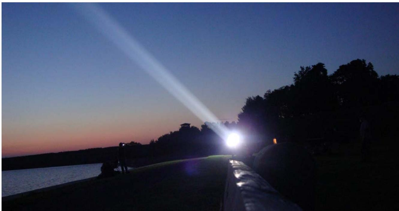
The intensity of the light is so powerful that looking directly into the light can result in burning of the retina of the eye. The flame from the carbon arc is visible in the photo below. The principles which cause the light to engage operate much like an arc welder. The light is reflected from a 5-foot diameter concave mirror and projected outward.
