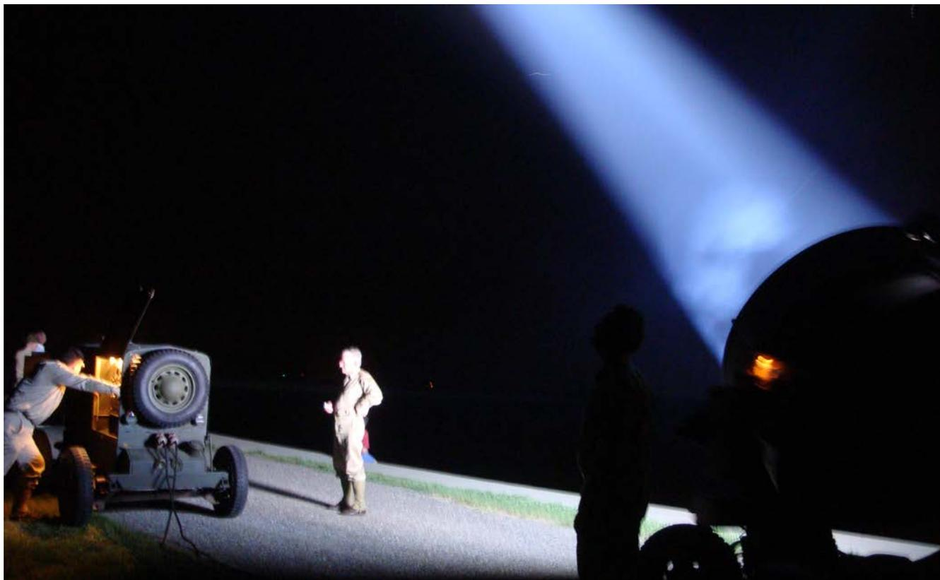
The searchlight works by burning carbon rods. Below, the white hot flame is clearly visible.
