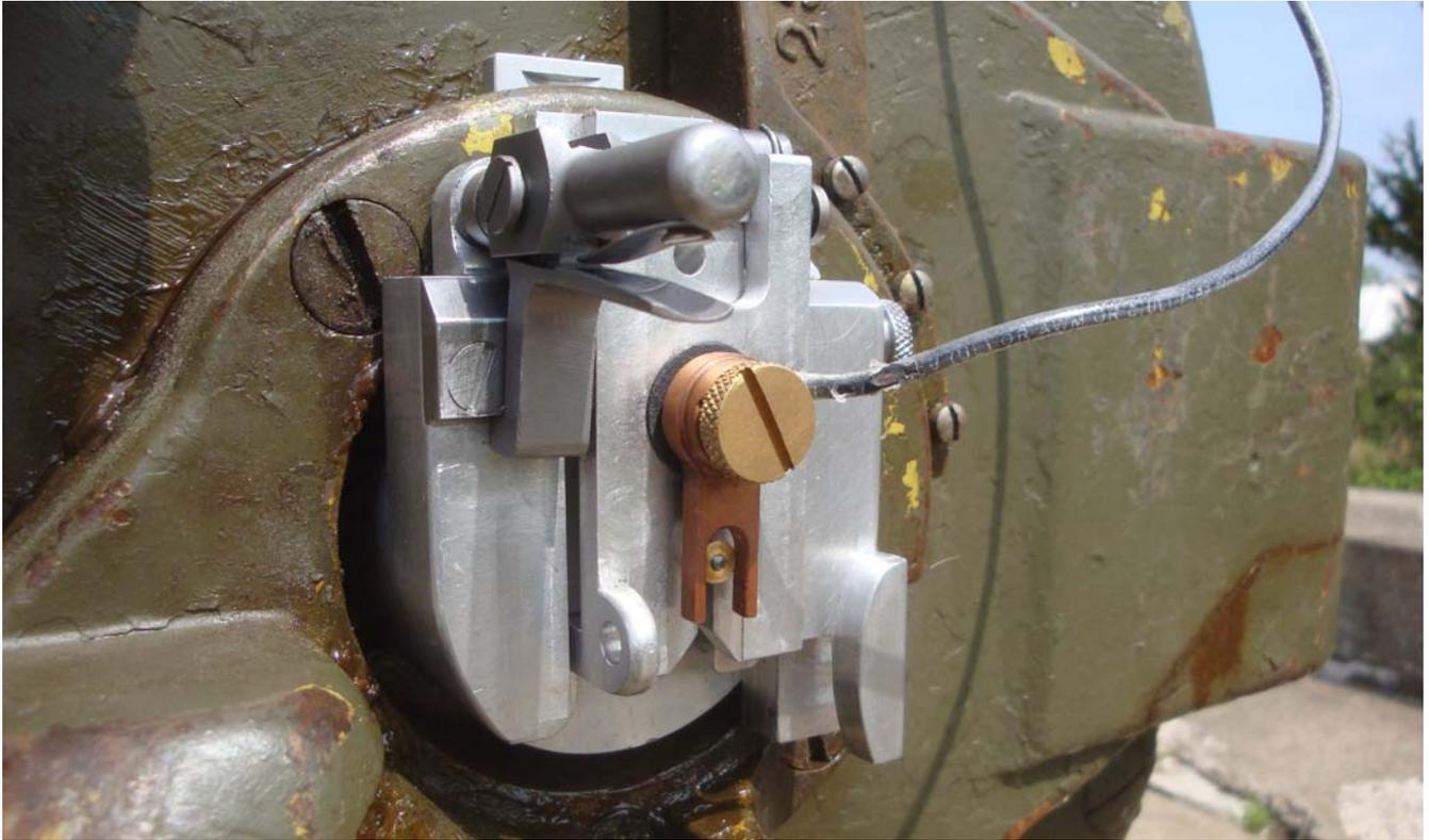
The device below is shown 'open,' with the "primer" partially extracted. These are specially produced primers designed to complete an electric circuit. Once we have perfected the reliability of these primers to complete an electric circuit, we will use them to complete a circuit for an audible "boom". Next step, figuring out the best way to produce that "boom". Any ideas?
