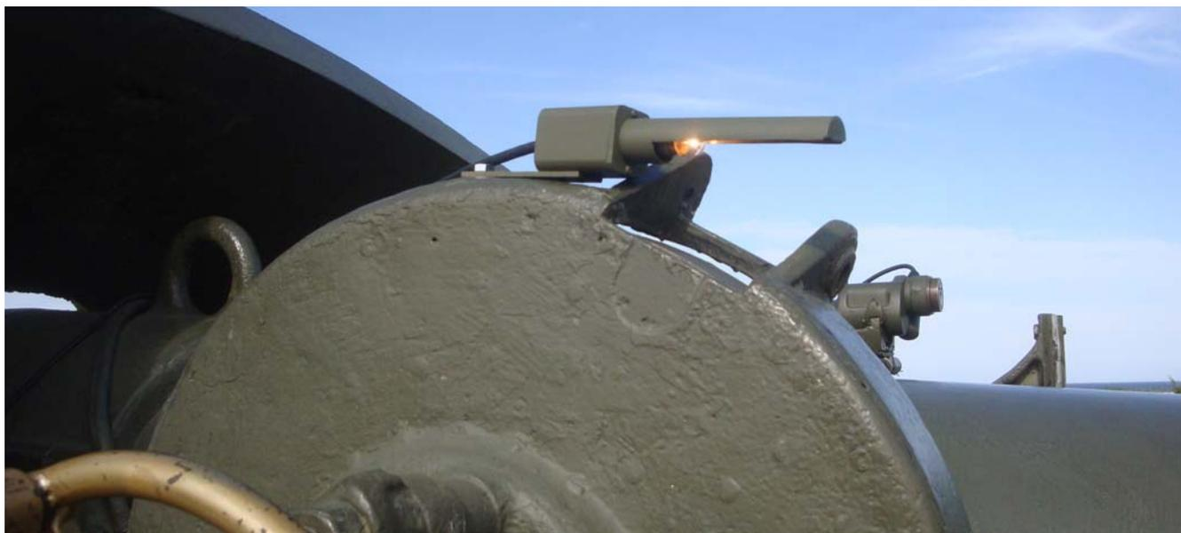
There were several other lights that needed to be made as well. Below, the newly fabricated light for the M1904 sight cradle elevation disk is shown.
