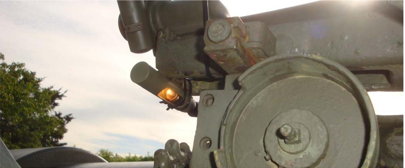
Looking from the gun pointers position, one can see the electric cable for the M1904 sight cradle light and the reticle light on the M1904 telescopic sight. The reticle is the vertical line inside the sight which is used to accurately track a target (in this case ships). This is the first time lights have been on this carriage since 1948, a remarkable milestone in the Battery's restoration.
