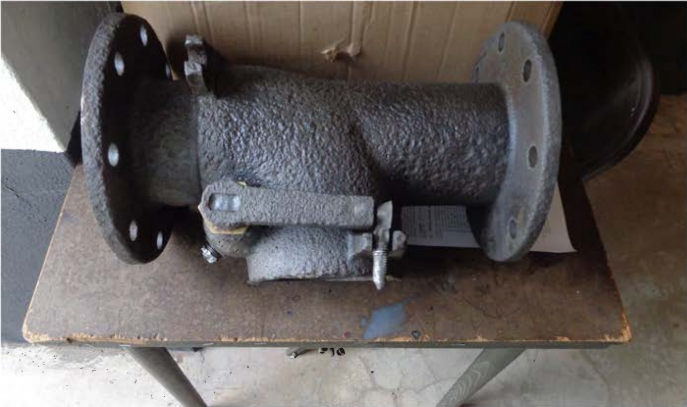
In the photo below the valve arm is shown in the closed position.
