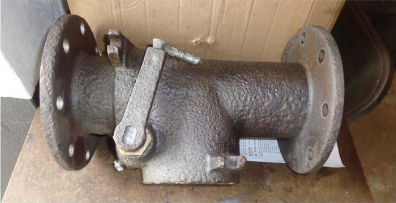
In the photo below the valve arm is shown in the closed position.
